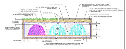
THE CHAMBERS SHALL BE DESIGNED AND TESTED IN ACCORDANCE WITH ASTM F2787 "STANDARD PRACTICE FOR STRUCTURAL DESIGN OF THERMOPLASTIC CORRUGATED WALL STORMWATER COLLECTION CHAMBERS". THE LOAD CONFIGURATION SHALL INCLUDE:
