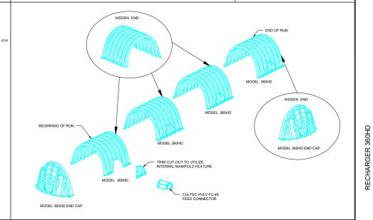
CULTEC RECHARGER 360HD CHAMBER STORAGE = 10.00 CF/FT [0.93 m<sup>3</sup>/m]
