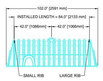
INSTALLED LENGTH ADJUSTMENT = 1.5' [0.46 m] ALL RECHARGER 330XLHD HEAVY DUTY UNITS ARE MARKED WITH A COLORED STRIPE FORMED INTO THE PART ALONG THE LENGTH OF THE CHAMBER.
