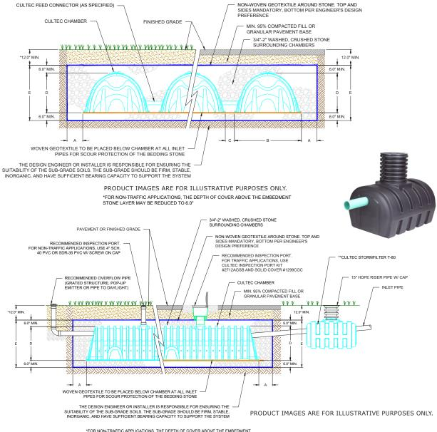
"FOR NON-TRAFFIC APPLICATIONS, THE DEPTH OF COVER ABOVE THE EMBEDMENT STONE LAYER MAY BE REDUCED TO 6.0" "CULTEC RECOMMENDS THE USE OF THE STORMFILTER T-80 UPSTREAM OF ALL SYSTEM INLETS. THE STORMFILTER T-80 MUST BE LOCATED IN A NON-TRAFFIC AREA
