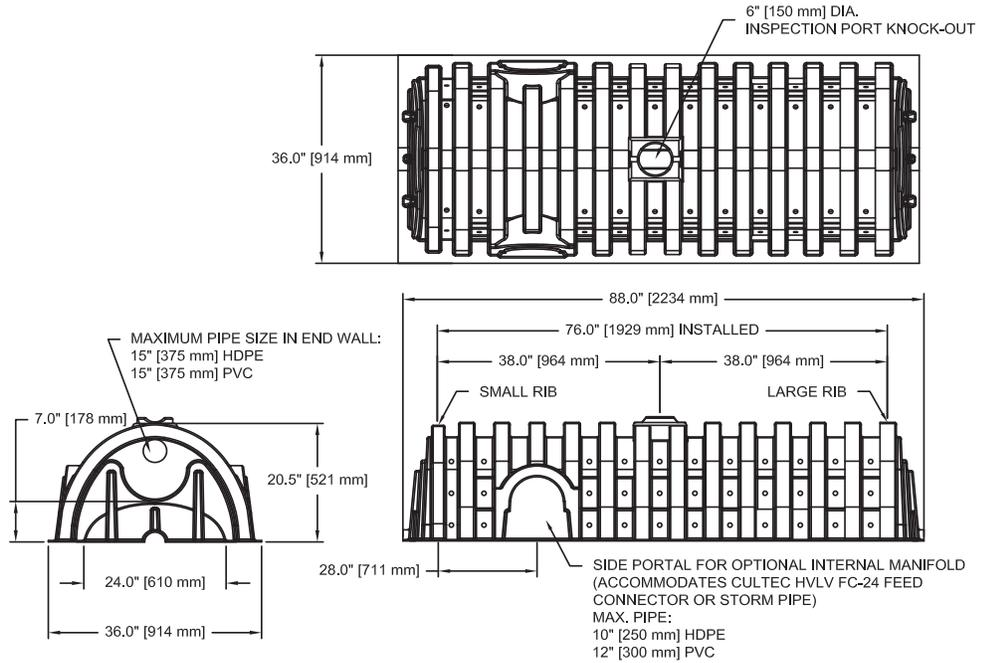
CULTEC RECHARGER 180HD CHAMBER STORAGE = 3.445 FT<sup>3</sup> / FT (0.32 M<sup>3</sup> / M)
