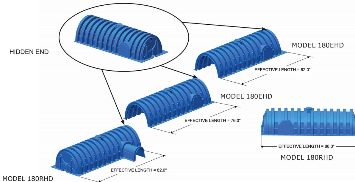
SHOWN WITH SIDE PORTAL TRIMMED AND OPTIONAL CULTREC HVLV FC-24 FEED CONNECTOR INSERTED.
