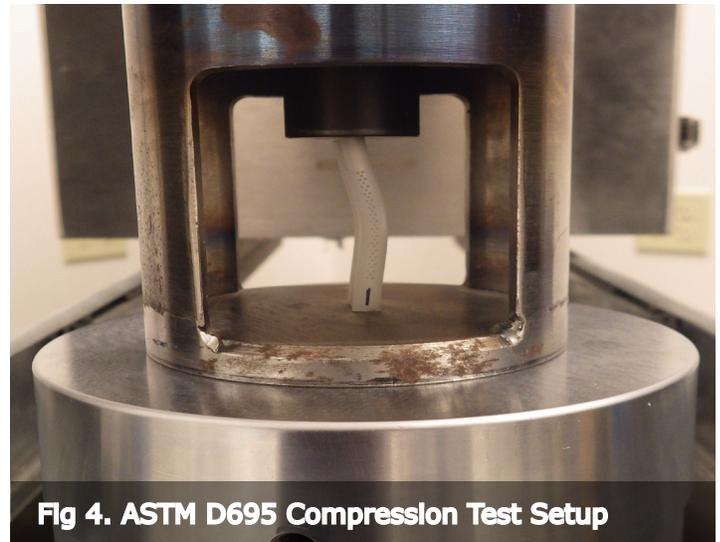
**Fig 4. ASTM D695 Compression Test Setup**
