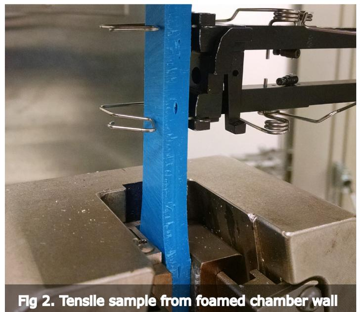
**Fig 2. Tensile sample from foamed chamber wall**
