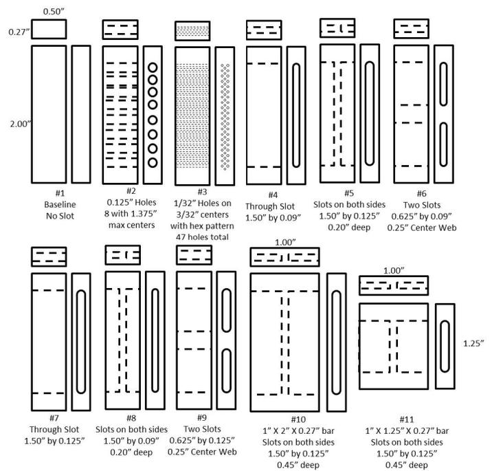
**Fig 3. Compression test sample configurations**
