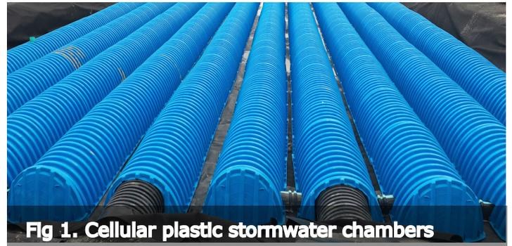
**Fig 1. Cellular plastic stormwater chambers**
