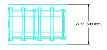
CULTEC HVLV F-110x4 FEED CONNECTOR CHAMBER STORAGE = 1.968 CF/FT (0.1828 m3/m) ALL HVLV F-110x4 UNITS ARE MARKED WITH A COLOR STRIPE FORMED INTO THE PART ALONG THE LENGTH OF THE CHAMBER.
