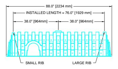
INSTALLED LENGTH ADJUSTMENT = 1.0' (0.3 m) ALL RECHARGER 180HD HEAVY DUTY UNITS ARE MARKED WITH A COLOR STRIPE FORMED INTO THE PART ALONG THE LENGTH OF THE CHAMBER.
